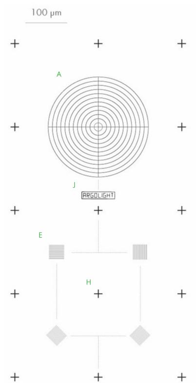
The maximum relative positioning error is  $\pm$  110 nm in XY and  $\pm$  110 nm in Z within each individual pattern. The thickness (in the Z direction) of these patterns is about (600  $\pm$  200) nm FWHM (Full Width at Half Maximum). Patterns description can be found below.
