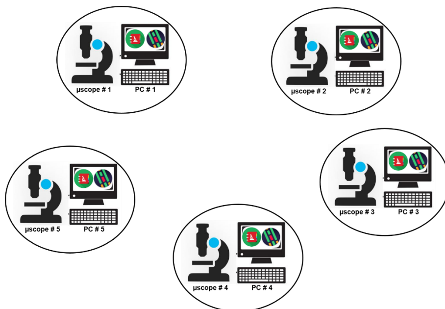
Figure 5: Sketch describing the deployed use of Daybook Data Manager for an example of five monitored microscopes. The images are saved in the computers driving the microscopes, where they are processed with Daybook Analysis. The generated quality data are afterwards managed in Daybook Data Manager in each local computer.
