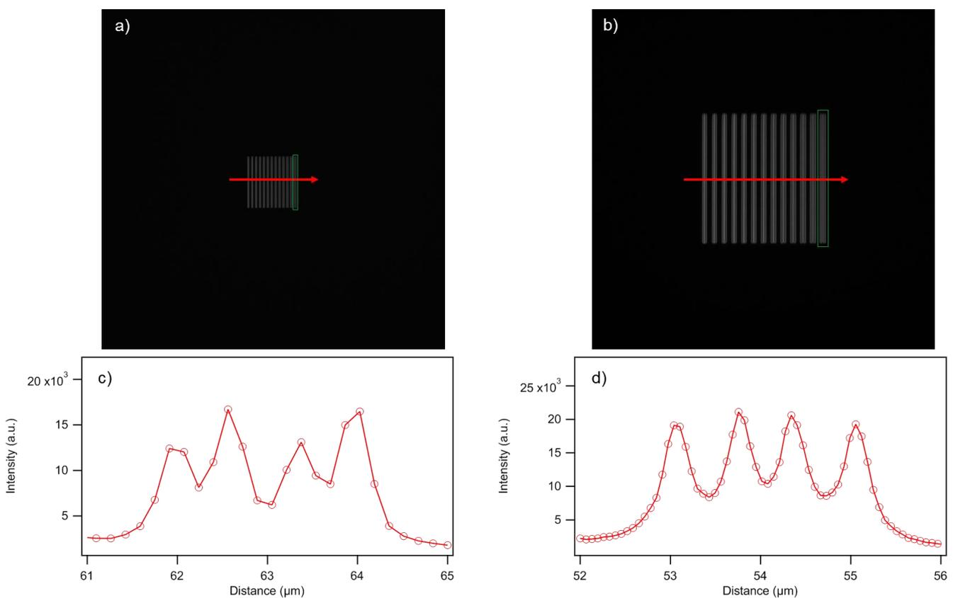
**Figure 10:** Images of a “gradually spaced lines” pattern acquired with the 40×/0.95 dry objective (a) and the 100×/1.46 oil objective (b), with their respective intensity line profiles perpendicular to the lines (c) and (d).
