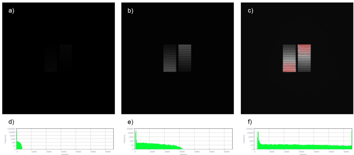
**Figure 8:** Images of a “2×16 intensity gradation” pattern acquired with the same illumination power and different exposure times, as well as their associated histograms (logarithmic scale). The exposure time increases from left to right; it was set too low on the left, appropriate in the middle and too high on the right. The saturated pixels are shown in red in the image on the right.
