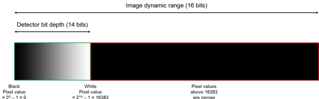
**Figure 9:** A 14-bit grayscale ranging from black (with the pixel value at 0) to white (with the pixel value at 16383). All the pixel values above 16383 are zeroes, to fill out the image 16-bit container. The useful part of the information in the image dynamic range is in the green rectangle, while the non-useful part is in the red one.
