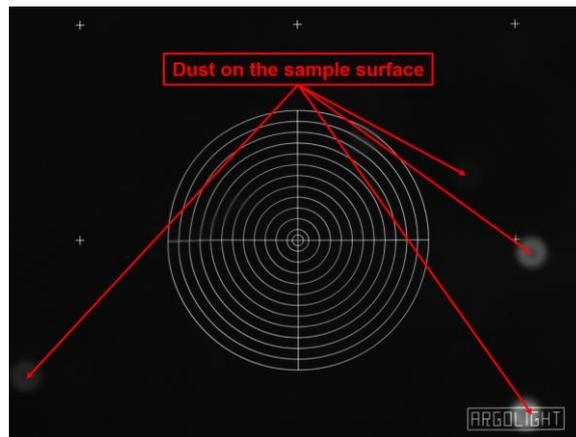
Figure 1: Image example of a sample with dust at the surface, inducing blurry spots in the image.
