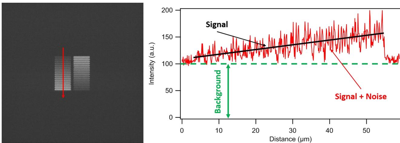
**Figure 7:** Images of a “2×16 intensity gradation” pattern (left) acquired at low illumination power and exposure time, and intensity profile (right) corresponding to the red line showing the signal, noise and background.
