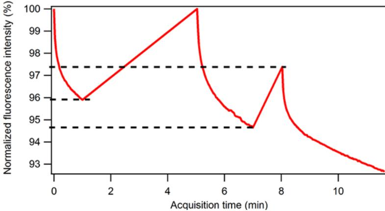
Fig.7: Typical fluorescence intensity recovery signal of the patterns. The power density was about 10 W.cm<sup>-2</sup>, the excitation wavelength was (470 ± 20) nm and the collection window was (525 ± 25) nm. After one minute of acquisition and four minutes of waiting time, the fluorescence fully recovers for these irradiation conditions. When the waiting time is not sufficient, the fluorescence intensity does not restart at its original level.
