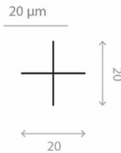
Fig. 16: Schematics of one of the repositioning crosses. All dimensions are in  $\mu\text{m}$ .
