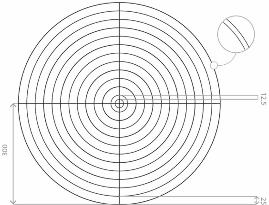
Fig.8: Schematics of the target. All dimensions are in  $\mu\text{m}$ .
