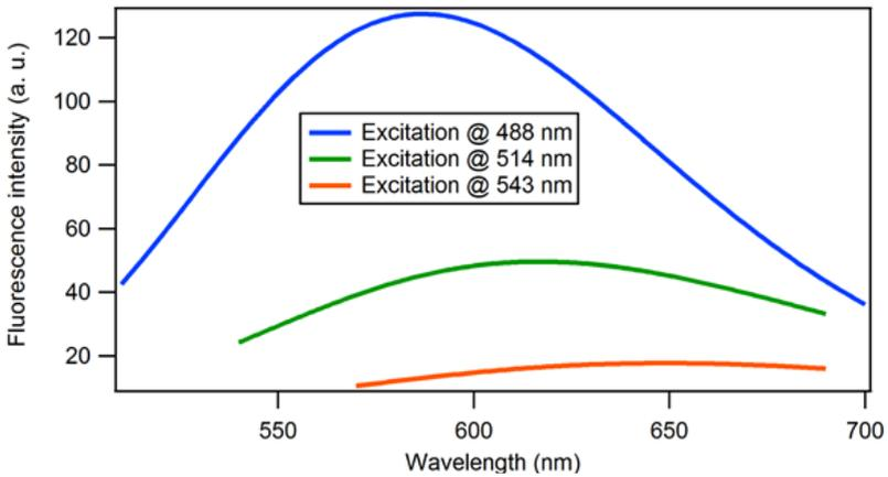
Fig.5: Typical emission spectra of the patterns for excitation wavelengths at 488, 514 and 543 nm.
