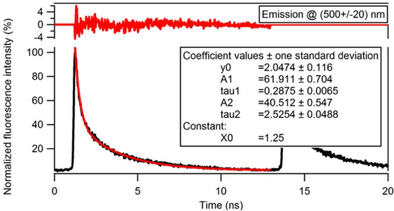
Fig.6: Typical fluorescence decay of the patterns for  $\lambda_{exc}=400$  nm,  $\Delta\lambda_{em}=500\pm 20$  nm, 10x/0.25 objective.
