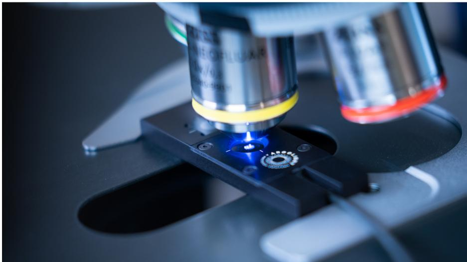
Fig.20:Argo-POWER<sup>HM</sup> head inserted in the sample holder of an upright wide-field fluorescence microscope.
