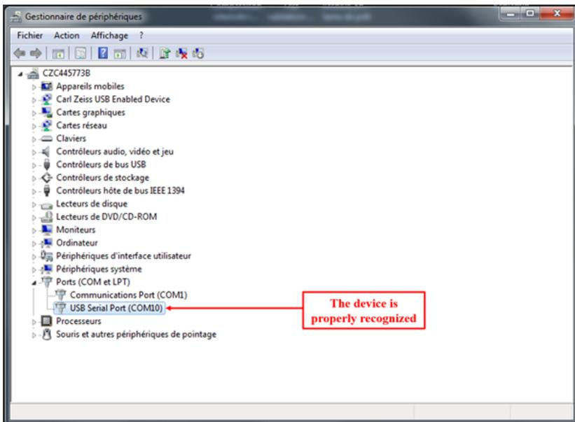
Fig.31: Device manager window showing the device is properly recognized by the PC.
