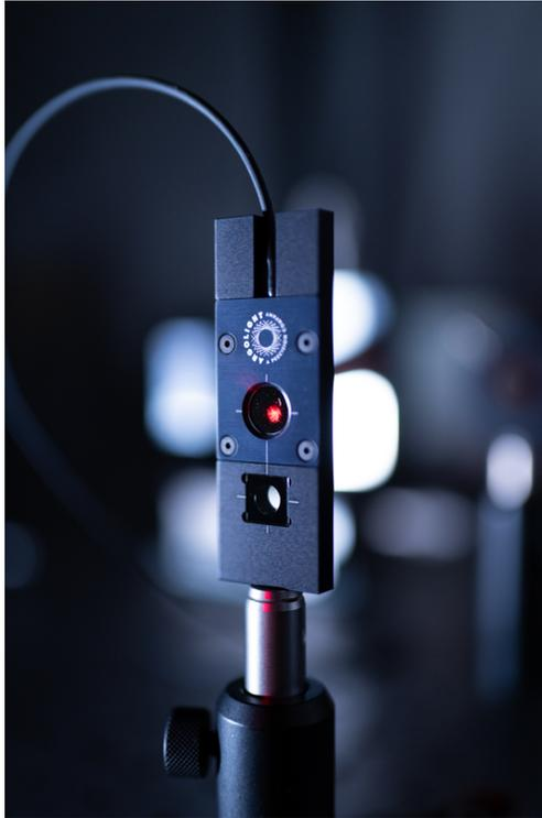
Fig.22: Argo-POWER<sup>HM</sup> head inserted across the optical path of a collimated light beam.
