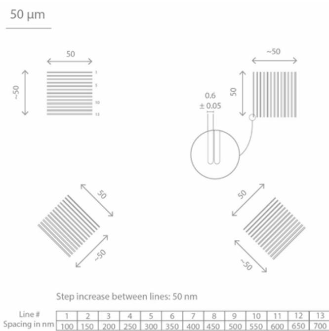
Fig.12: Schematics of the vertical, horizontal and  $\pm 45^\circ$ -oriented gradually spaced lines. All dimensions are in  $\mu\text{m}$ .
