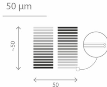
Fig. 11: Schematics of the  $2\times 16$  intensity gradation. All dimensions are in  $\mu\text{m}$ .
