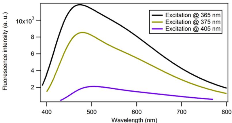
Fig.4: Typical emission spectra of the patterns for excitation wavelengths at 365, 375 and 405 nm.
