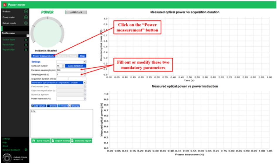
Fig.23: User interface for optical power measurement
