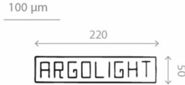
Fig.17: Schematics of the Argolight logo. All dimensions are in  $\mu\text{m}$ .
