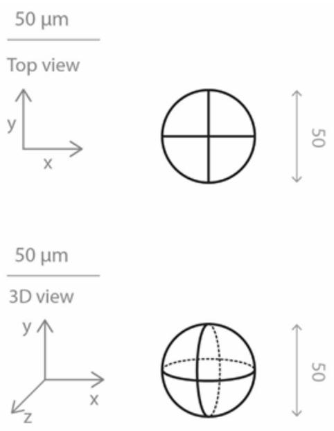
Fig.14: Schematics of the meridians of a sphere. All dimensions are in  $\mu\text{m}$
