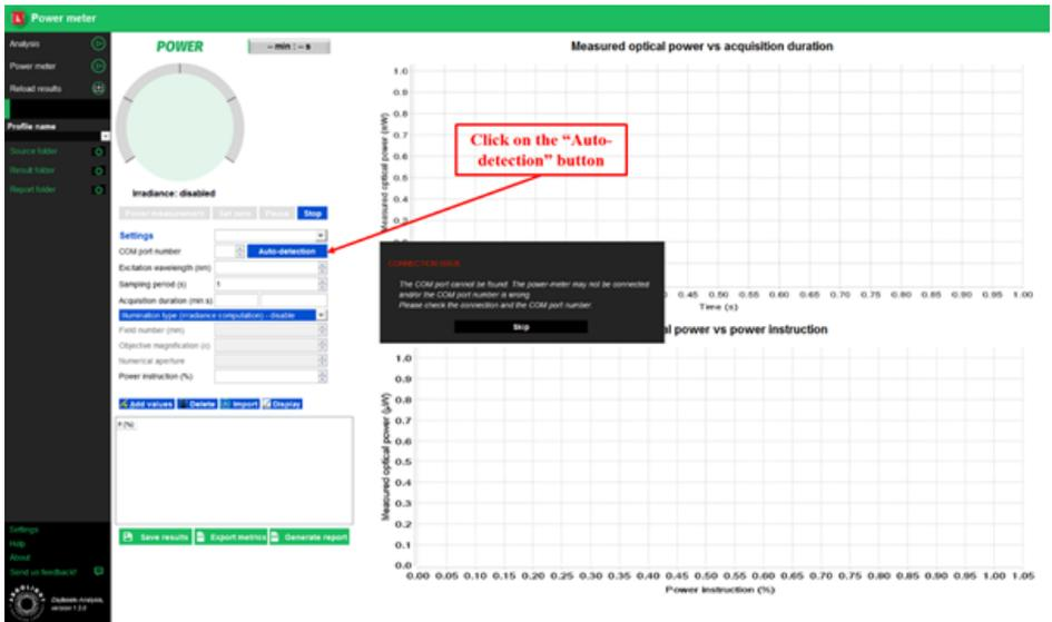
Fig.30: Displayed warning message for connection issues.
