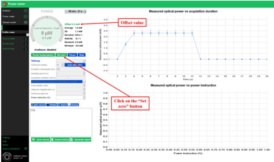
Fig.33: Offset option to subtract the optical power from any other contribution than the light source to be measured.
