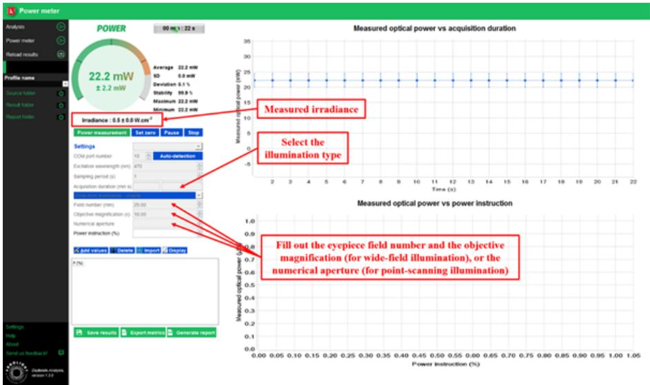
Fig.26: Example of irradiance live measurement for wide-field illumination.
