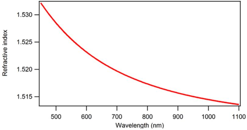
Fig.1: Dispersion of the refractive index of the glass.
