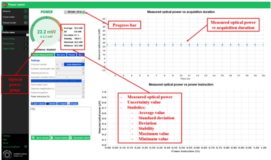
Fig.24: Live optical power measurement.
