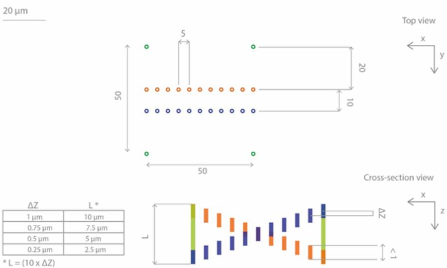
Fig.15: Schematics of the 3D crossing stairs. All dimensions are in  $\mu\text{m}$ .
