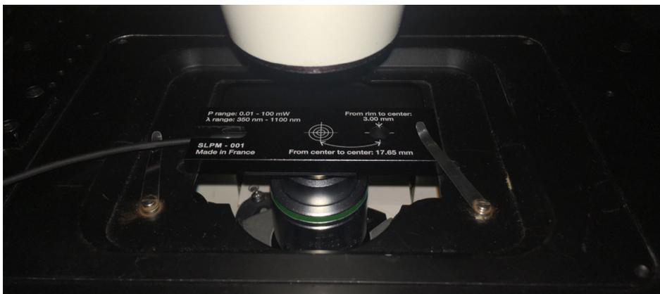
Fig.21:Argo-POWER<sup>HM</sup> head inserted in the sample holder of an inverted fluorescence microscope.
