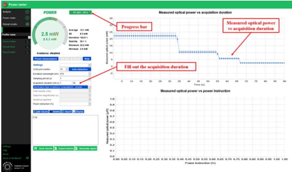
Fig.25: Example of evolution of the optical power versus the acquisition duration.
