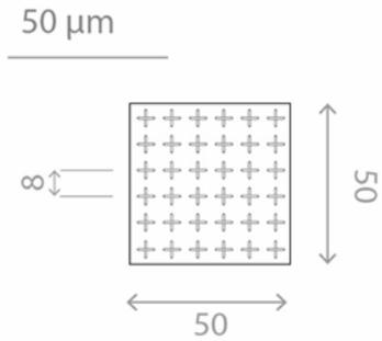
Fig.13: Schematics of the matrix of crosses. All dimensions are in  $\mu\text{m}$ .
