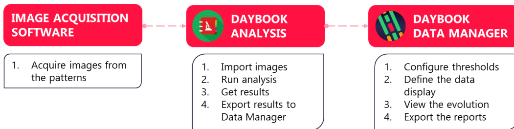
Figure 1: Schematics of the quality control workflow with Daybook Analysis and Daybook Data Manager.
